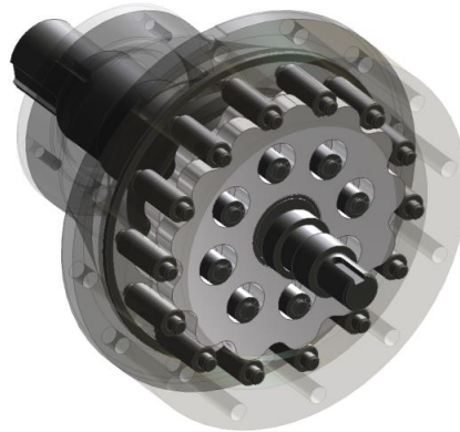
Figure 1. Model of cycloid drive
